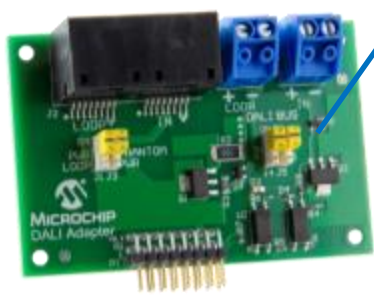
DALI Adapter with 2-wire & RJ45 connections
