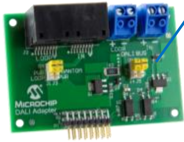
DALI Adapter with 2-wire & RJ45 connections
