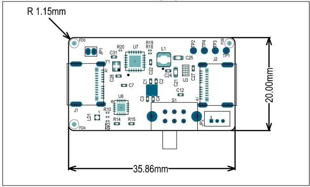
FIGURE C-6: EV23B43A ASSEMBLY DRAWING (BOTTOM)
