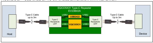
FIGURE 2-2: USE CASE UP TO 6m CABLE EXTENSION WITH REPEATER
