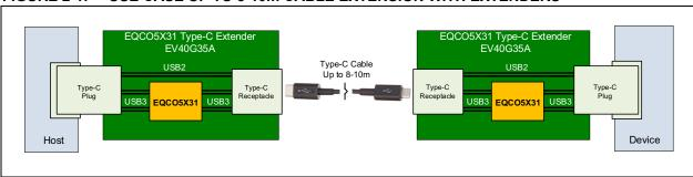
FIGURE 2-1: USE CASE UP TO 8-10m CABLE EXTENSION WITH EXTENDERS
