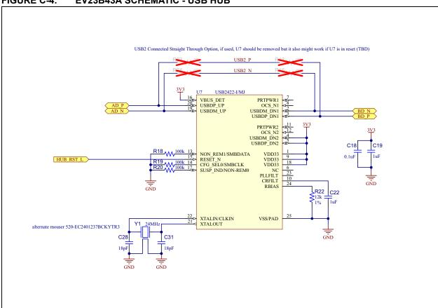
FIGURE C-4: EV23B43A SCHEMATIC - USB HUB
