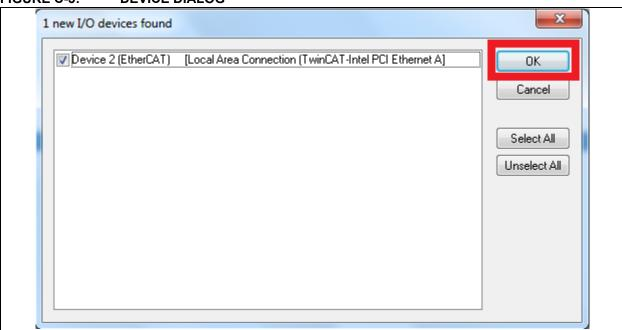
If the check box is not checked, as displayed in Figure C-4, then either the device is not functional or driver is not installed properly.
