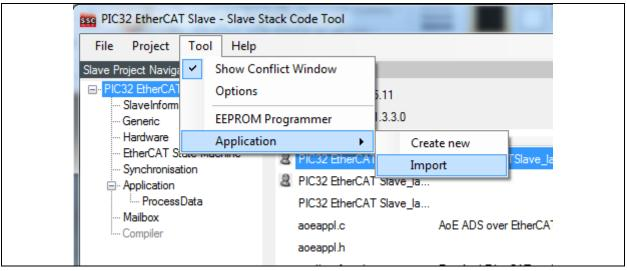
9. Select the file pic32\_mchp\_gpio\_sample\_app.xlsx which can be found in the directory {SDK\_INSTALL\_PATH}/EVB-LAN9252\_SDK\_VX.X\EVB-LAN9252-3PORT\_PIC32\_SDK\_VX.X/. pic32\_mchp\_gpio\_sample\_app.xlsx is an object file which contains the information about application objects information.
