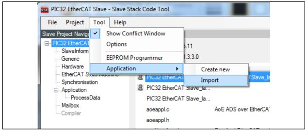
7. Select the file pic32\_mchp\_gpio\_sample\_app.xlsx which can be found in the directory {SDK\_INSTALL\_PATH}/EVB- LAN9252\_SDK\_VX.X\EVB-LAN9252-4PORT\_PIC32\_SD-K VX.X/.
