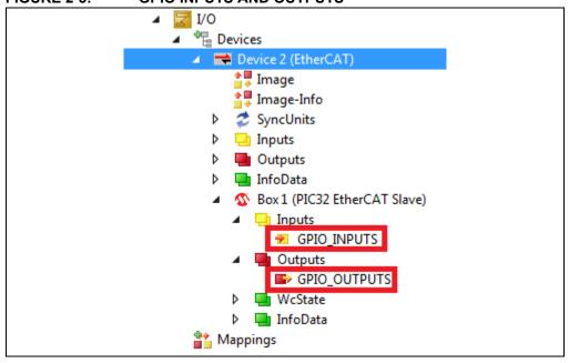
2. As part of this demo, two object variables GPIO\_INPUTS and GPIO\_OUTPUTS are mapped to PIC32 GPIOs as mentioned below.
