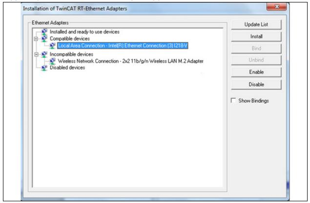
5. Once the TwinCAT driver is installed successfully, the driver is compatible with the TwinCAT master. The network adapter will then be moved to "Installed and ready to use devices" as displayed in
