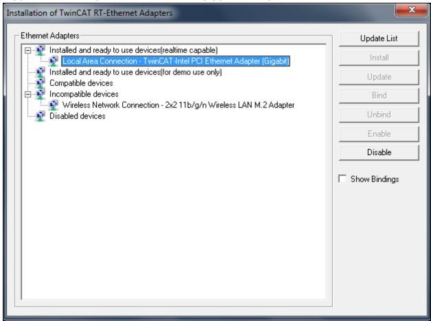
6. Go to the corresponding network adapter properties and then select TwinCAT drivers as displayed in Figure A-5 and Figure A-6.
