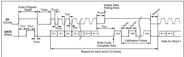
Note 1: S0 and S1 button inputs to be held to ground during the entire programming sequence.
