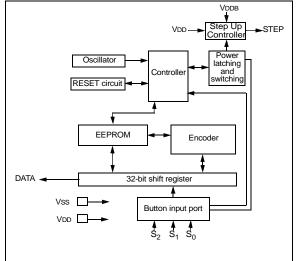
The HCS201 combines a 32-bit hopping code, generated by a nonlinear encryption algorithm, with a 28-bit serial number and 6 information bits to create a 66-bit code word. The code word length eliminates the threat of code scanning and the code hopping mechanism makes each transmission unique, thus rendering code capture and resend schemes useless.
