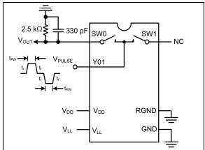
FIGURE 3-6: Tx Pulse Width.
