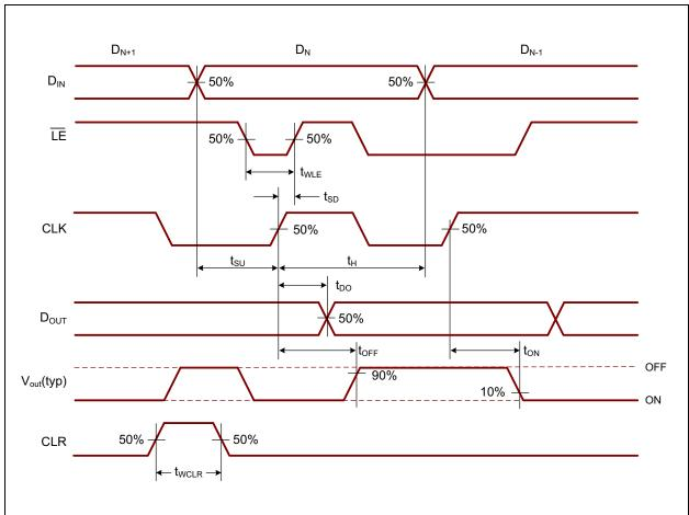
FIGURE 1-1: Logic Input Timing Diagram.
