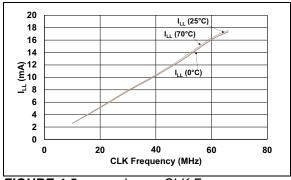
FIGURE 4-5: I<sub>LL</sub> vs. CLK Frequency.
