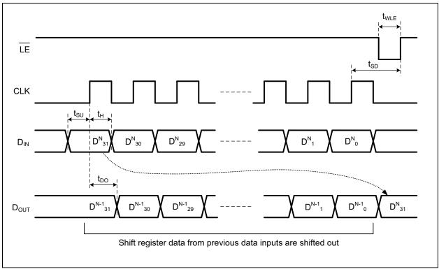
FIGURE 5-2: Latch Enable Timing Diagram.
