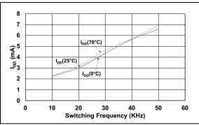
**FIGURE 4-2:** I<sub>DD</sub> vs. Switching Frequency.
