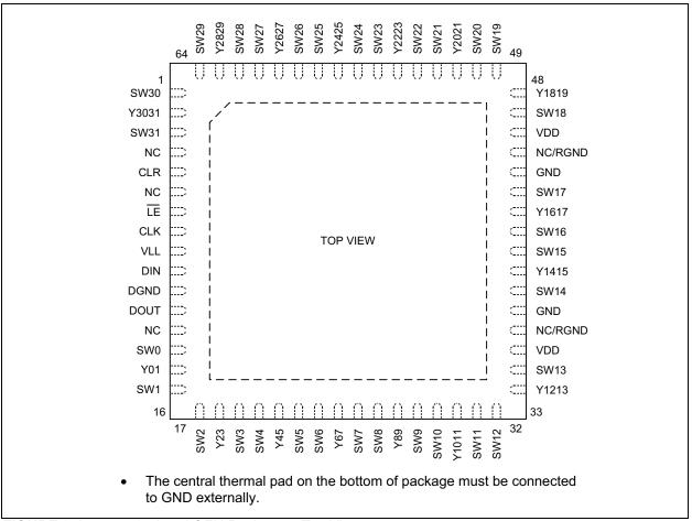
FIGURE 2-1: 64-Lead QFN Package – Top View.
