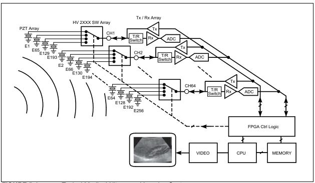
FIGURE 5-1: Typical Medical Ultrasound Imaging System.
