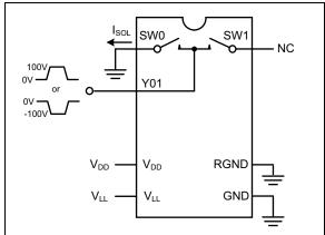
FIGURE 3-1: Switch-Off Leakage per Switch.
