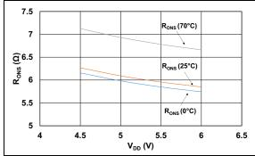
FIGURE 4-1: R<sub>ONS</sub> at 5 mA vs. V<sub>DD</sub>.
