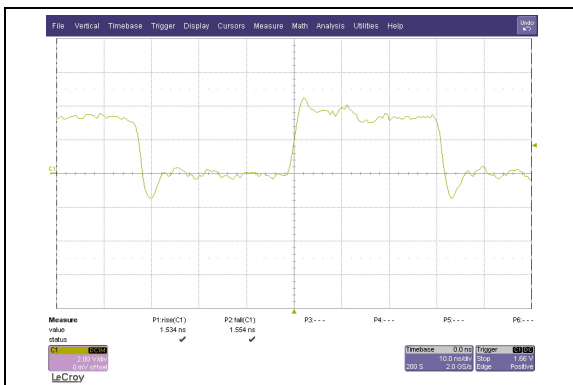
FIGURE 1-20: Typical SDO output Rise Time and Fall Time
