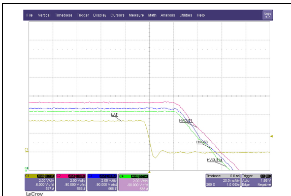
FIGURE 1-18: Typical LATCHC to HV OUT Propagation Delay
