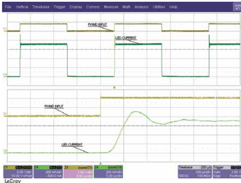
Fig. 3. PWM Dimming – Rising Edge Waveform
