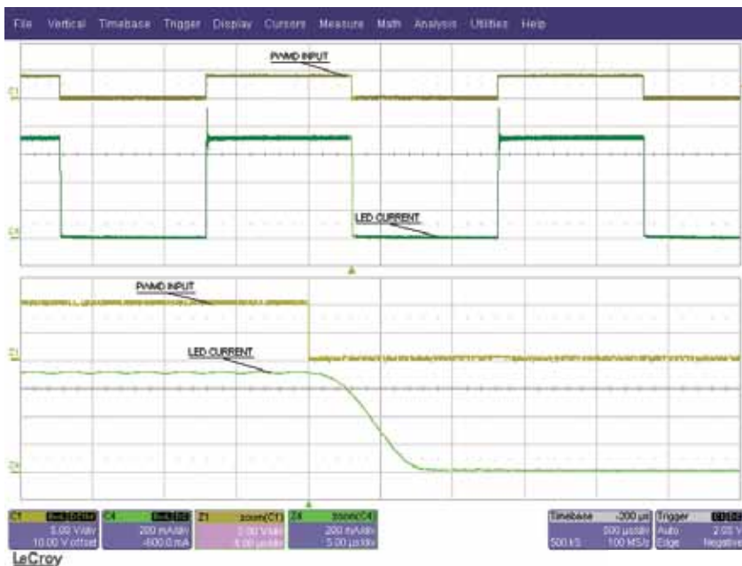
Fig. 4. PWM Dimming – Falling Edge Waveform
