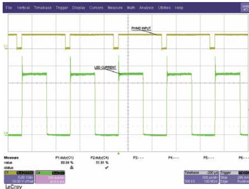
Fig. 6. PWM Dimming of LED current with 2.78k between NTC and GND
