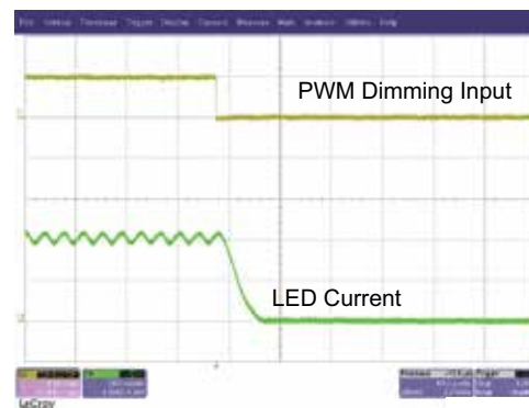
(c) PWM Dimming Fall Time Time Scale : 10µs/div
