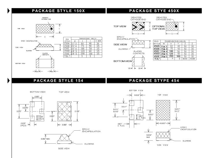
Packages are designed with wrap-around metalized castellations for superior assembly results.
