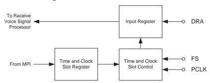
Figure 4. Receive PCM Interface
