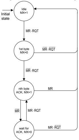
Figure 11. Monitor Transmitter Mode Diagram
