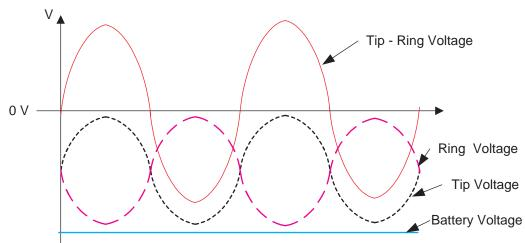
Figure 17. Balanced Ringing with Fixed Supply
