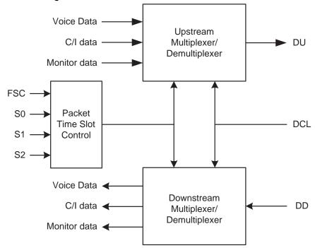
Figure 8. GCI Interface and Packet Time Slot Selection
