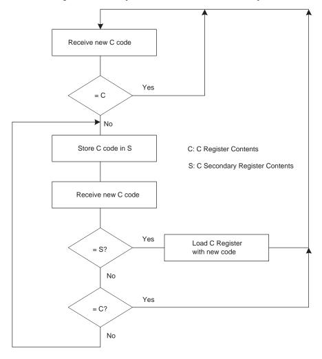
Figure 9. Security Procedure For C Downstream Byte
