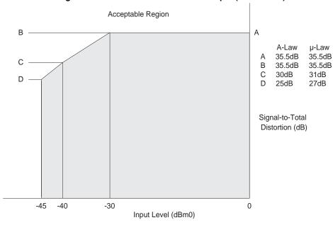
Figure 30. Total Distortion with Tone Input (Both Paths)
