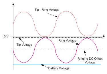
Figure 19. Unbalanced Ringing with Fixed Supply
