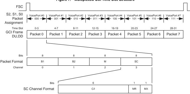
Figure 7. Multiplexed GCI Time Slot Structure
