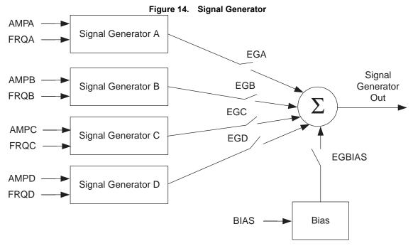
Signal Generator A is used for ringing signal generation and is automatically enabled when entering the ringing state. It can produce sinusoidal or trapezoidal signals. When generating a trapezoid, Signal Generator B is not available and some of its parameters are used to configure the trapezoid. For more details on trapezoidal ringing, see the Trapezoidal Ringing Application Note (Document ID #081476).
