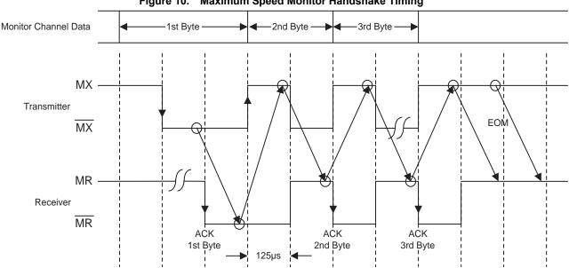
Figure 10. Maximum Speed Monitor Handshake Timing
