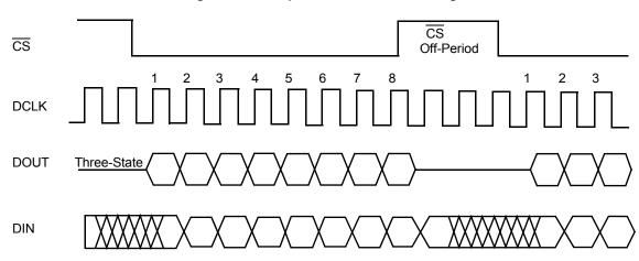
Figure 6. Microprocessor Interface Timing
