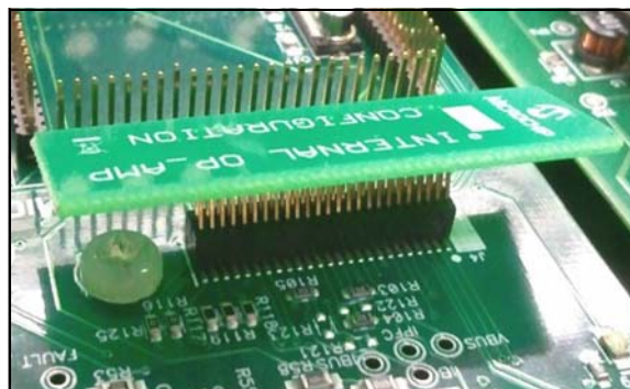
FIGURE 2: INTERNAL OP AMP CONFIGURATION BOARD
