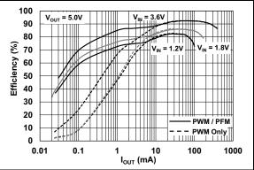
**FIGURE 2-6:** 5.0V V<sub>OUT</sub> PFM/PWM Mode Efficiency vs. I<sub>OUT</sub>.
