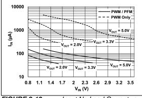
FIGURE 2-13: Input No Load Current vs. V<sub>IN</sub>.
