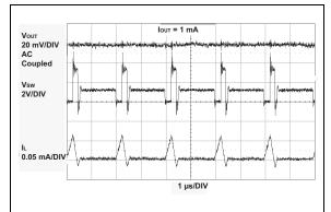
FIGURE 2-17: MCP1640B 3.3V V<sub>OUT</sub> PWM Mode Waveforms.
