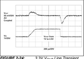
**FIGURE 2-24:** 3.3V V<sub>OUT</sub> Line Transient Waveforms.
