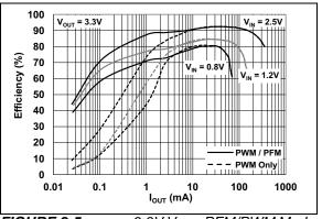
**FIGURE 2-5:** 3.3V V<sub>OUT</sub> PFM/PWM Mode Efficiency vs. I<sub>OUT</sub>.
