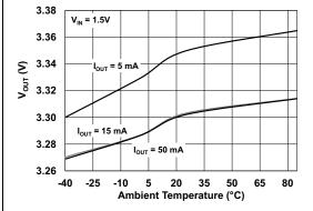
FIGURE 2-8: 3.3V V<sub>OUT</sub> vs. Ambient Temperature.
