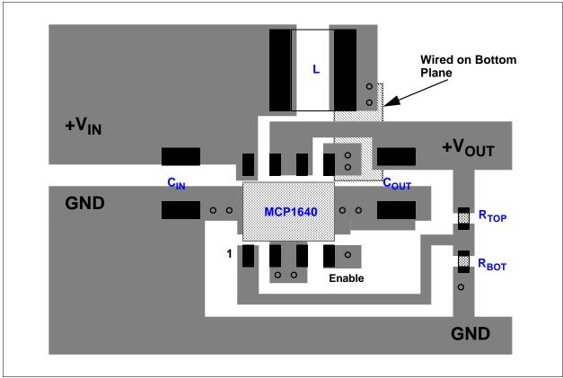
FIGURE 5-2: MCP1640/B/C/D DFN-8 Recommended Layout.
