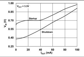
FIGURE 2-10: Minimum Start-Up and Shutdown V<sub>IN</sub> into Resistive Load vs. I<sub>OUT</sub>.
