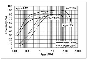
FIGURE 2-4:2.0V V<sub>OUT</sub> PFM/PWM ModeEfficiency vs. I<sub>OUT</sub>.
