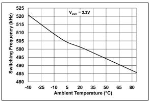
FIGURE 2-11: F<sub>OSC</sub> vs. Ambient Temperature.
