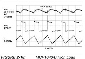
FIGURE 2-18: MCP1640/B High Load Waveforms.
