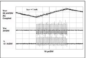
FIGURE 2-16:MCP1640 3.3V V<sub>OUT</sub> PFMMode Waveforms.
