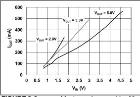
**FIGURE 2-3:** Maximum I<sub>OUT</sub> vs. V<sub>IN</sub> After Start-Up, V<sub>OUT</sub> 10% Below Regulation Point.
