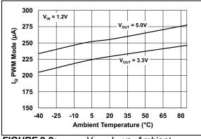
**FIGURE 2-2:** V<sub>OUT</sub> I<sub>Q</sub> vs. Ambient Temperature in PWM Mode.
