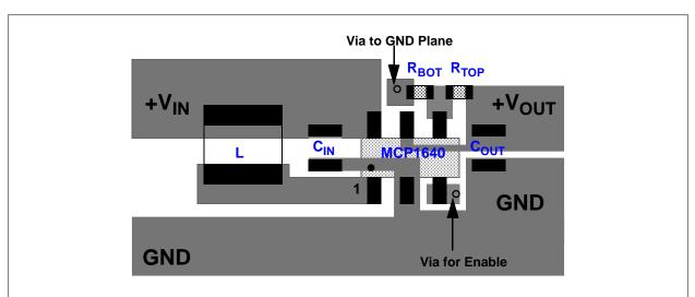
FIGURE 5-1: MCP1640/B/C/D SOT-23-6 Recommended Layout.
