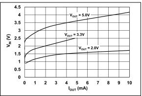
**FIGURE 2-12:** PWM Pulse-Skipping Mode Threshold vs. IOUT.
