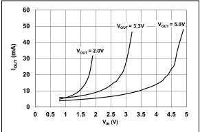
**FIGURE 2-15:** Average of PFM/PWM Threshold Current vs. V<sub>IN</sub>.
