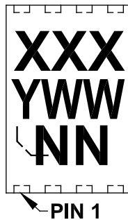
8-Lead TDFN (2x3x0.75 mm)
