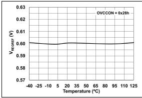
**FIGURE 7-8:**  $V_{REGREF}$  vs. Temperature  $(V_{REGREF} = 0.6V)$ .
