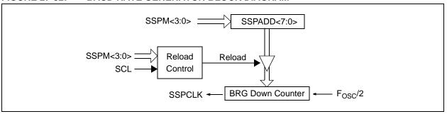
**Note:** Values of 0x00, 0x01 and 0x02 are not valid for SSPADD when used as a Baud Rate Generator for I<sup>2</sup>C. This is an implementation limitation.
