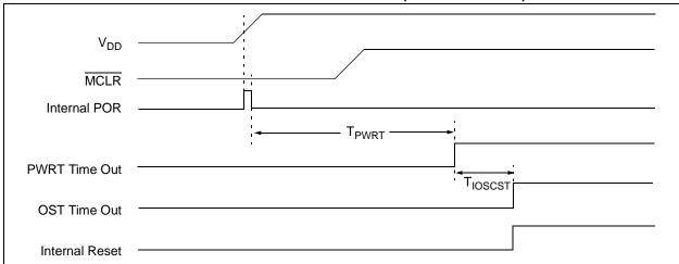
FIGURE 14-4: TIME-OUT SEQUENCE ON POWER-UP (DELAYED MCLR): CASE 2
