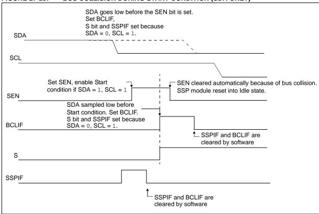
FIGURE 27-26: BUS COLLISION DURING START CONDITION (SCL = 0)
