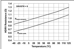
**FIGURE 7-13:** HDRV R<sub>DSon</sub> vs. Temperature.
