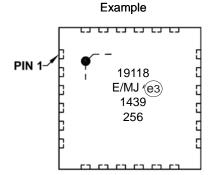
28-Lead QFN (5x5x0.9 mm) (MCP19119 only)
