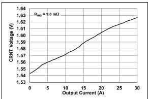
FIGURE 7-17: CRNT Voltage vs. Output Current.
