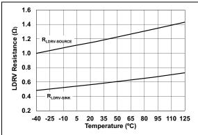
**FIGURE 7-15:** LDRV R<sub>DSon</sub> vs. Temperature.
