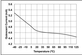
**FIGURE 7-1:**  $I_O$  vs. Temperature.
