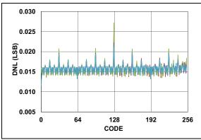
FIGURE 7-3: OVCCON DAC DNL vs. Code and Temperature (-40°C to +125°C).
