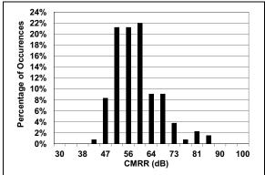
FIGURE 7-18: Remote Sense Amplifier CMRR.
