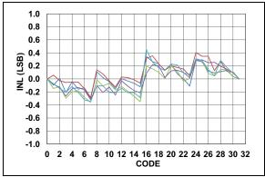
FIGURE 7-4: OVFCON DAC INL vs. Code and Temperature (-40°C to +125°C).
