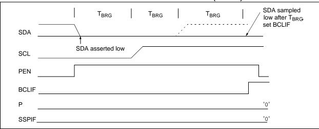
FIGURE 27-31: BUS COLLISION DURING A STOP CONDITION (CASE 2)
