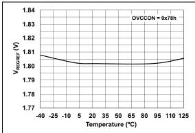
**FIGURE 7-9:**  $V_{REGREF}$  vs. Temperature  $(V_{REGREF} = 1.8V)$ .
