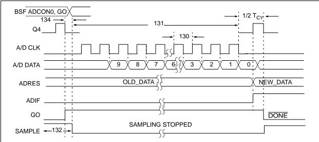
**Note 1:** If the A/D clock source is selected as RC, a time of T<sub>CY</sub> is added before the A/D clock starts. This allows the SLEEP instruction to be executed.
