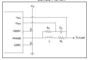
The value of  $R_S$  and  $C_S$  can be found by using Equation 3-3. When the current sense filter time constant is set equal to the inductor time constant, the voltage appearing across  $C_S$  approximates the current flowing in the inductor, multiplied by the inductor resistance.
