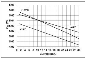
FIGURE 7-7: V<sub>DD</sub> vs. Output Current.
