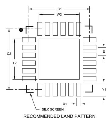
Units MILLIMETERS **Dimension Limits** MIN MOM MAX Contact Pitch Ε 0.50 BSC Optional Center Pad Width W2 2.60 Optional Center Pad Length T2 2.60 Contact Pad Spacing C1 3.90 C2 Contact Pad Spacing 3.90 X1 0.30 Contact Pad Width Contact Pad Length Y1 0.85
