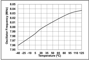
FIGURE 7-16: Oscillator Frequency vs. Temperature.
