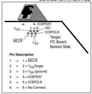
Another connector often found in use with the PICkit<sup>™</sup> programmers is a standard 6-pin header with 0.1 inch spacing. Refer to Figure 28-2.
