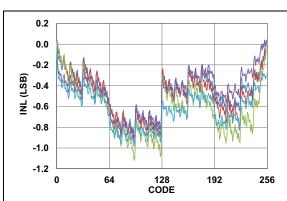
FIGURE 7-2: OVCCON DAC INL vs. Code and Temperature (-40°C to +125°C).
