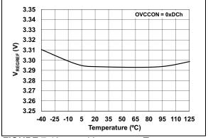
**FIGURE 7-10:**  $V_{REGREF}$  vs. Temperature  $(V_{REGREF} = 3.3V)$ .
