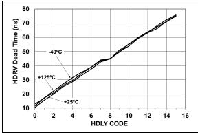
FIGURE 7-11: HDRV Dead Time vs. HDLY Code.
