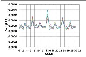
FIGURE 7-5: OVFCON DAC DNL vs. Code and Temperature (-40°C to +125°C).
