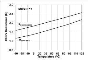
**FIGURE 7-14:** HDRV R<sub>DSon</sub> vs. Temperature.
