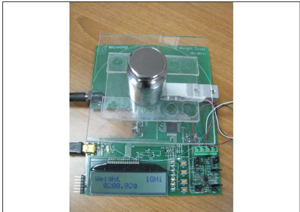
FIGURE 1-1: MCP3421 Weight Scale Demo Board.
