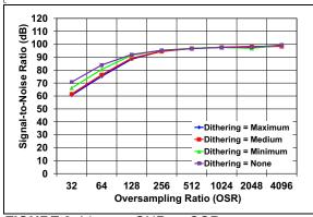
FIGURE 2-14: SNR vs.OSR.
