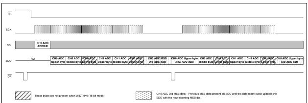
FIGURE 6-6: Typical Continuous Read Communication (SPI Mode 0,0).
