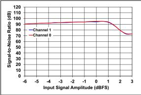
FIGURE 2-25: SNR vs. Input Signal Amplitude.
