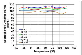
FIGURE 2-30: SFDR vs. Temperature.
