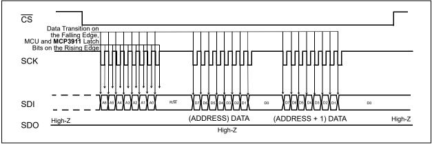
FIGURE 6-3: Device Write (SPI Mode 1,1 – SCK Idles High).
