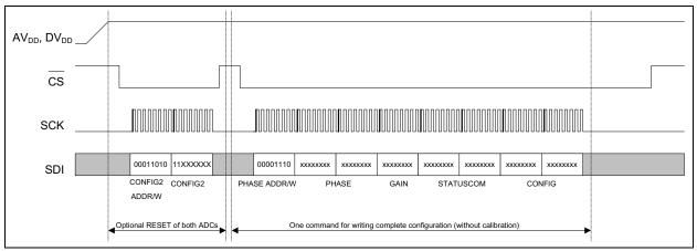
FIGURE 6-8: Recommended Configuration Sequence at Power-up.
