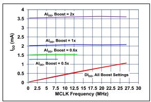
**FIGURE 2-41:** Operating Current vs. MCLK,  $V_{DD} = 2.7V$ .
