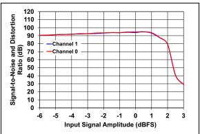
FIGURE 2-24: SINAD vs. Input Signal Amplitude.
