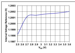
FIGURE 2-36: Internal Voltage Reference vs. Supply Voltage.
