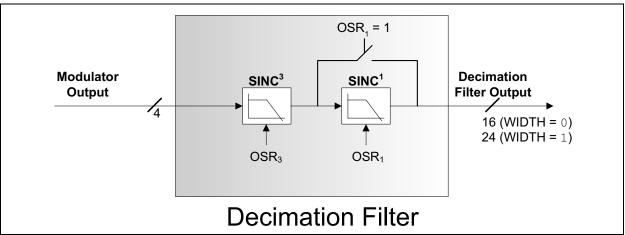
FIGURE 5-3: MCP3911 Decimation Filter Block Diagram.
