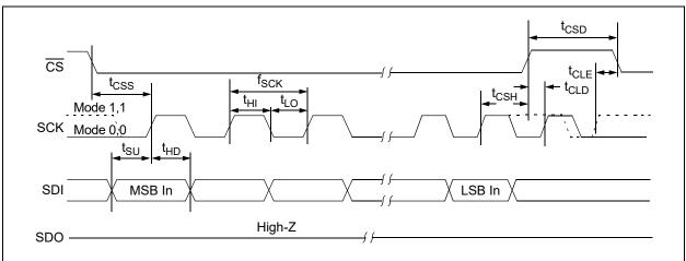
FIGURE 1-2: Serial Input Timing Diagram.
