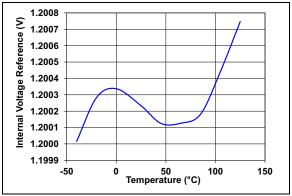
**FIGURE 2-35:** Internal Voltage Reference vs. Temperature.
