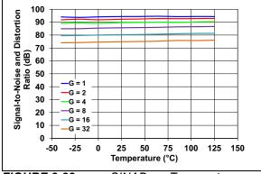
FIGURE 2-28: SINAD vs. Temperature.
