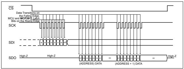
FIGURE 6-2: Device Read (SPI Mode 1,1 – SCK Idles High).
