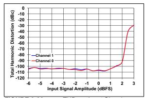
FIGURE 2-23: THD vs. Input Signal Amplitude.
