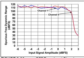
**FIGURE 2-26:** SFDR vs. Input Signal Amplitude.
