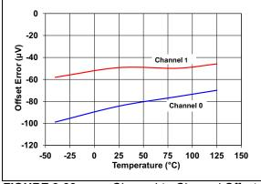
**FIGURE 2-33:** Channel-to-Channel Offset Match vs. Temperature.
