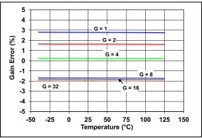
FIGURE 2-34: Gain Error vs. Temperature.
