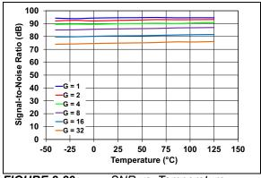
FIGURE 2-29: SNR vs. Temperature.
