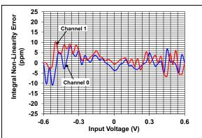
FIGURE 2-38: Integral Nonlinearity (Dithering Maximum).
