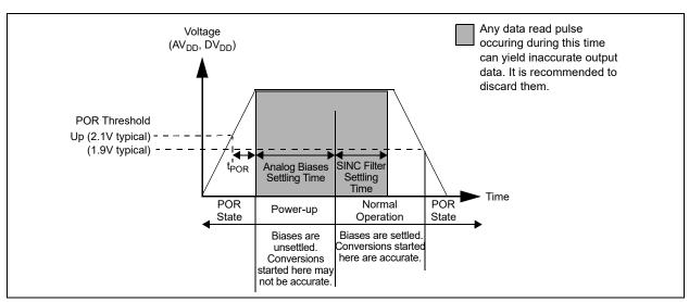
FIGURE 5-7: Power-on Reset Operation.
