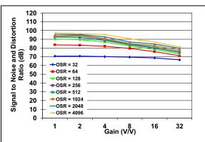
FIGURE 2-21: SINAD vs. GAIN (Dithering Off).
