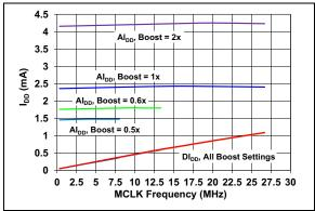
**FIGURE 2-40:** Operating Current vs. MCLK,  $V_{DD} = 3.3V$ .
