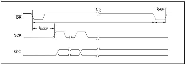
FIGURE 1-3: Data Ready Pulse/Sampling Timing Diagram.
