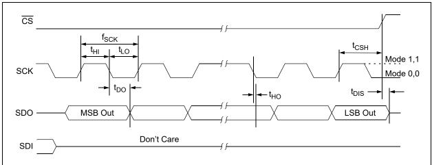
FIGURE 1-1: Serial Output Timing Diagram.
