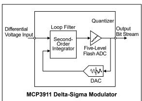
**FIGURE 5-1:** Simplified Delta-Sigma ADC Block Diagram.
