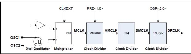
FIGURE 4-1: Clock Sub-Circuitry.
