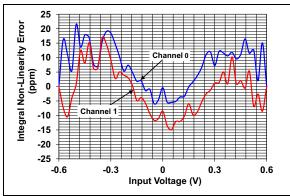
FIGURE 2-39: Integral Nonlinearity (Dithering Off).
