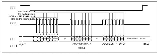
FIGURE 6-5: Device Write (SPI Mode 0,0 – SCK Idles Low).
