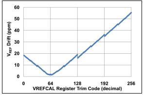
**FIGURE 5-6:** V<sub>REF</sub> Tempco vs. V<sub>REFCAL</sub> Trim Code Chart.
