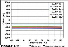
FIGURE 2-33: Offset vs. Temperature vs. Gain.
