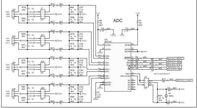
FIGURE 7-1: MCP3912 Application Example Schematic.
