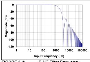
**FIGURE 5-3:** SINC Filter Frequency Response, OSR = 256, MCLK = 4 MHz, PRE[1:0] = 00.
