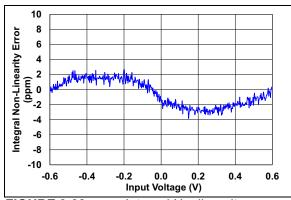
FIGURE 2-38: Integral Nonlinearity (Dithering Maximum).
