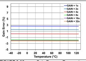
FIGURE 2-35: Gain Error vs. Temperature vs. Gain.
