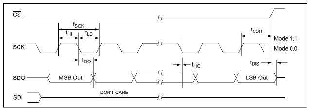
FIGURE 1-1: Serial Output Timing Diagram.
