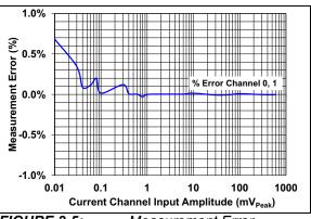
**FIGURE 2-5:** Measurement Error with 1-Point Calibration.
