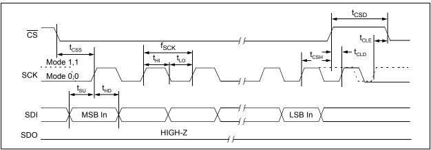
FIGURE 1-2: Serial Input Timing Diagram.
