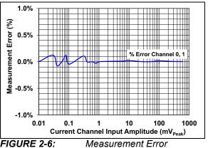
FIGURE 2-6: Measurement I with 2-Point Calibration.
