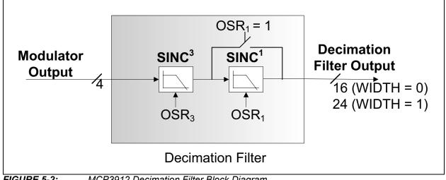
FIGURE 5-2: MCP3912 Decimation Filter Block Diagram.
