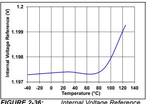
**FIGURE 2-36:** Internal Voltage Reference vs. Temperature.
