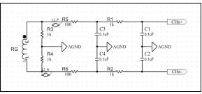
*FIGURE 7-7:* Second-Order Anti-Aliasing Filter for Rogowski Coil-Based Designs.
