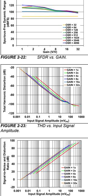
FIGURE 2-24: SINAD vs. Input Signal Amplitude.
