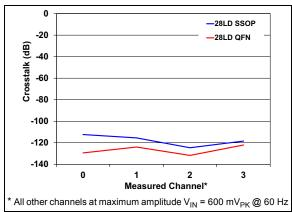
FIGURE 2-32: Crosstalk vs. Measured Channel.
