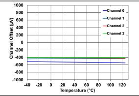
**FIGURE 2-34:** Channel Offset Matching vs. Temperature.
