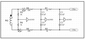
FIGURE 8-7: Second-Order Anti-Aliasing Filter for Rogowski Coil-Based Designs.
