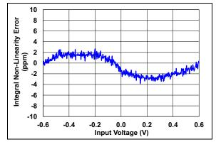
FIGURE 2-36: Integral Nonlinearity (Dithering Maximum).
