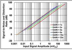
FIGURE 2-24: SINAD vs. Input Signal Amplitude.
