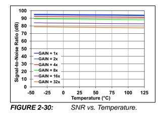
Note: Unless otherwise indicated,  $AV_{DD} = 3V$ ;  $DV_{DD} = 3V$ ;  $T_A = +25$  °C; MCLK = 4 MHz; PRESCALE = 1; OSR = 256; GAIN = 1; Dithering = Maximum;  $V_{IN} = -0.5$  dBFS @ 60 Hz on all channels; VREFEXT = 0; CLKEXT = 1; BOOST[1:0] = 10.
