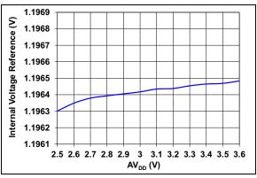
FIGURE 2-35: Internal Voltage Reference vs. Supply Voltage.
