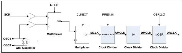
FIGURE 4-1: Clock Sub-Circuitry.
