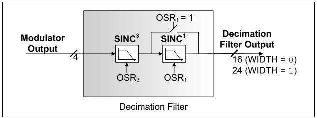
FIGURE 5-3: MCP3918 Decimation Filter Block Diagram.
