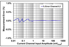
FIGURE 2-6:Measurement Error with2-Point Calibration.
