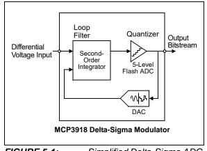
FIGURE 5-1: Block Diagram. Simplified Delta-Sigma ADC
