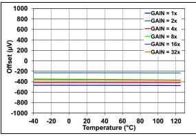
FIGURE 2-32: Offset vs. Temperature vs. Gain.
