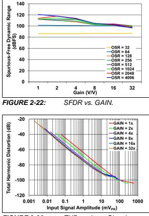
THD vs. Input Signal **FIGURE 2-23:** Amplitude.
