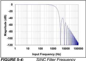
**FIGURE 5-4:** SINC Filter Frequency Response, OSR = 256, MCLK = 4 MHz, PRE[1:0] = 00.
