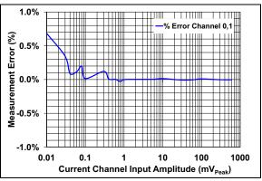
*FIGURE 2-5:* Measurement Error with 1-Point Calibration.
