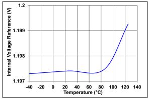
FIGURE 2-34: Internal Voltage Reference vs. Temperature.
