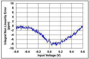
FIGURE 2-39: Integral Nonlinearity (Dithering Off).
