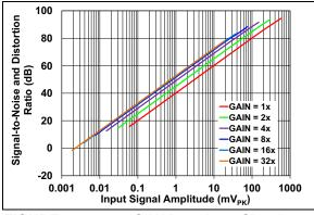
FIGURE 2-24: SINAD vs. Input Signal Amplitude.
