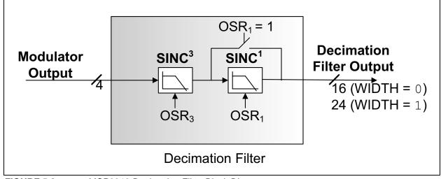
FIGURE 5-2: MCP3919 Decimation Filter Block Diagram.
