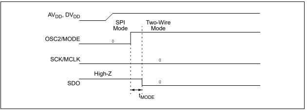
FIGURE 1-5: Entering Two-Wire Interface Mode Timing Diagram.
