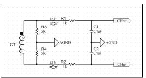
FIGURE 8-6: First-Order Anti-Aliasing Filter for CT-Based Designs.
