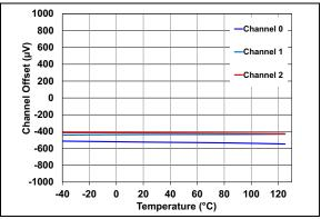
FIGURE 2-34: Channel Offset Matching vs. Temperature.
