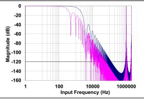
**FIGURE 5-4:** SINC Filter Frequency Response, OSR = 4096 (in pink), OSR = 512 (in blue), MCLK = 4 MHz, PRE[1:0] = 00.
