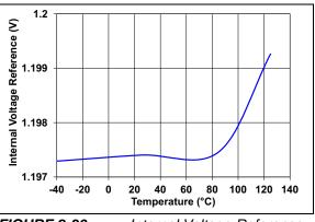
FIGURE 2-36: Internal Voltage Reference vs. Temperature.
