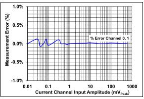
FIGURE 2-6:Measurement Error with2-Point Calibration.
