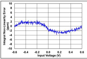
FIGURE 2-38: Integral Nonlinearity (Dithering Maximum).
