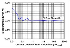
FIGURE 2-5:Measurement Error with1-Point Calibration.
