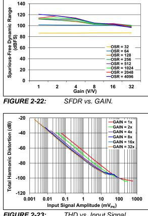
**FIGURE 2-23:** THD vs. Input Signal Amplitude.
