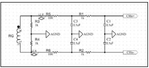
FIGURE 8-7: Second-Order Anti-Aliasing Filter for Rogowski Coil-Based Designs.
