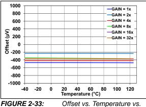
FIGURE 2-33: Offset vs. Temperature vs. Gain.
