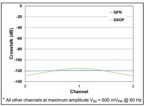
FIGURE 2-32: Crosstalk vs. Measured Channel.
