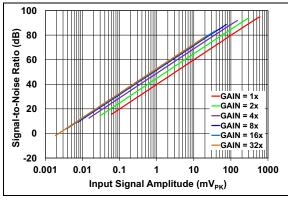
FIGURE 2-25: SNR vs. Input Signal Amplitude.
