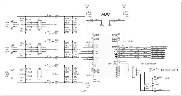
FIGURE 8-1: MCP3919 Application Example Schematic.
