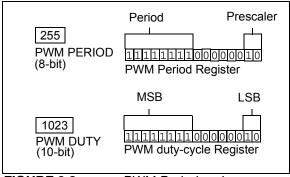
FIGURE 8-2: PWM Period and Duty-Cycle Registers.
