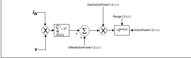
FIGURE 5-4: Channel 1 or Channel 2 Active Power Calculation Signal Flow.
