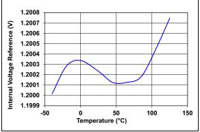
**FIGURE 2-10:** Internal Voltage Reference vs. Temperature.
