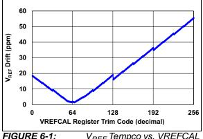
**FIGURE 6-1:** V<sub>REF</sub> Tempco vs. VREFCAL Trimcode Chart.
