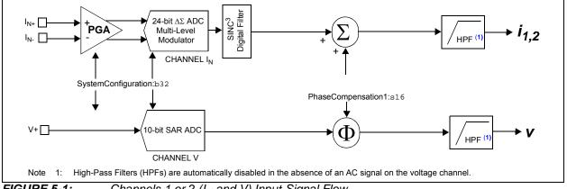
FIGURE 5-1: Channels 1 or 2 (I<sub>N</sub> and V) Input-Signal Flow.
