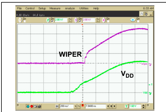
FIGURE 2-52: 50 k \Omega – Power-Up Wiper Response Time.
