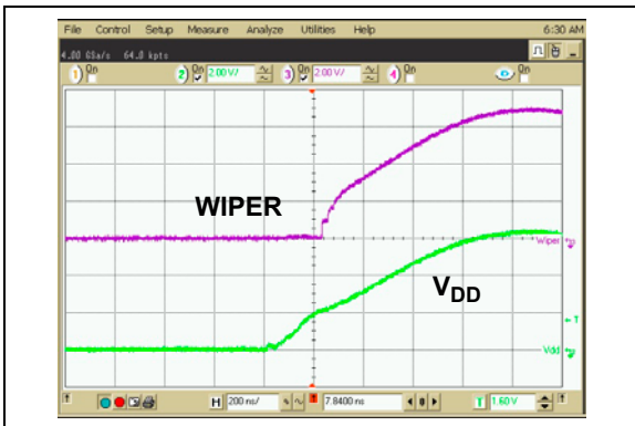
FIGURE 2-14: 2.1 kΩ – Power-Up Wiper Response Time.
