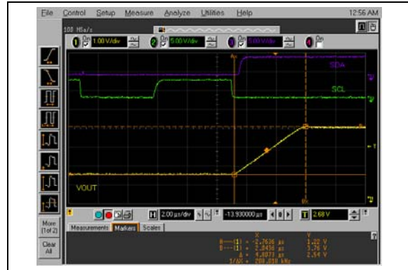
FIGURE 2-98: Half-Scale Settling Time (400h to C00h) (MCP4726).
