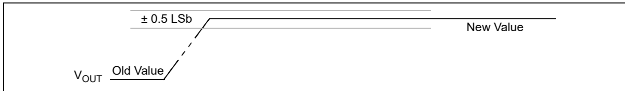
FIGURE 1-1: V_{OUT} Settling Time Waveforms.
