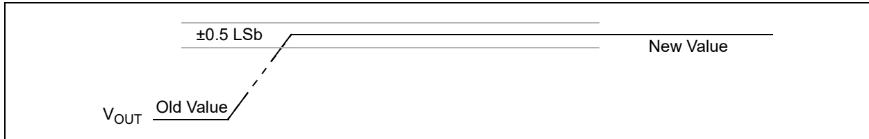
FIGURE 1-1: V_{OUT} Settling Time Waveforms.
