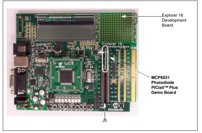
FIGURE 2-1: MCP6031 Photodiode PICtail<sup>™</sup> Plus Demo Board Set-Up.
