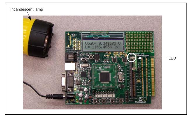
FIGURE 2-2: MCP6031 Photodiode PICtail<sup>™</sup> Plus Demo Board Operation.
