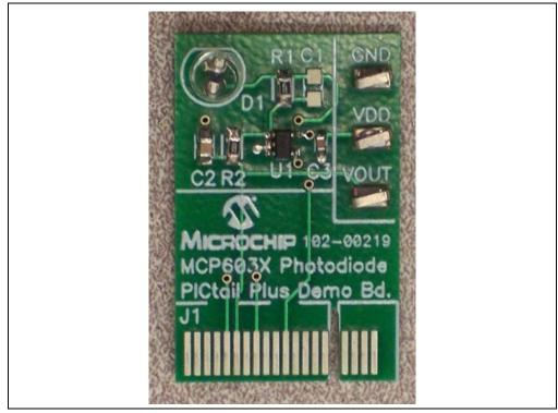
Figure 1-3 shows the top view of the MCP6031 Photodiode PICtail<sup>™</sup> Plus Demo Board.
