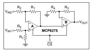
FIGURE 4-12: Difference Amplifier Circuit.
