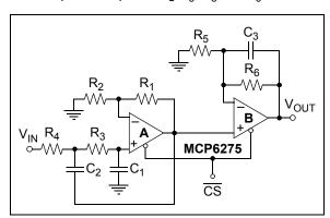
FIGURE 4-15: Second Order Sallen-Key Low-Pass Filter with an Extra Pole-Zero Pair and Chip Select.
