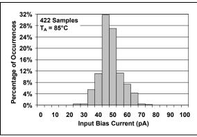
**FIGURE 2-2:** Input Bias Current at  $T_A = +85$ °C.
