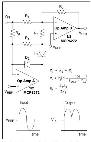
FIGURE 4-8: Active Full-wave Rectifier.
