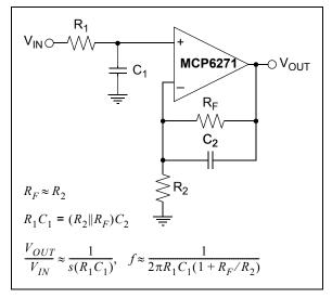
FIGURE 4-9: Non-Inverting Integrator.
