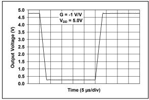
**FIGURE 2-29:** Large Signal Inverting Pulse Response.
