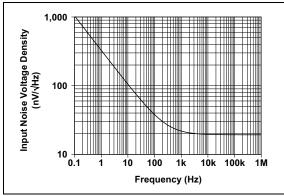
FIGURE 2-20: Input Noise Voltage Density vs. Frequency.
