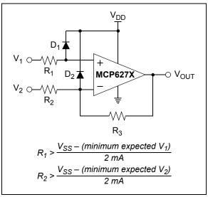
FIGURE 4-2: Protecting the Analog Inputs.
