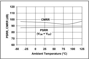
**FIGURE 2-12:** CMRR, PSRR vs. Temperature.
