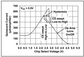
**FIGURE 2-28:** Quiescent Current vs. Chip Select (CS) Voltage, with  $V_{DD} = 5.5V$  (MCP6273 and MCP6275 only).
