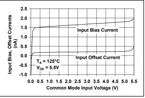
**FIGURE 2-16:** Input Bias, Offset Currents vs. Common-mode Input Voltage, with  $T_A = +125$ °C.
