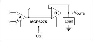
**FIGURE 4-10:** Isolating the Load with a Buffer.
