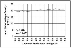
**FIGURE 2-23:** Input Noise Voltage Density vs. Common-mode Input Voltage, with f = 1 kHz.
