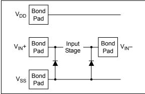
FIGURE 4-1: Simplified Analog Input ESD Structures.
