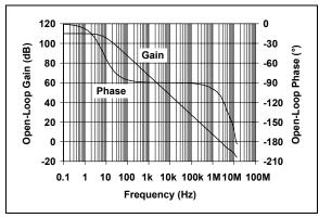
**FIGURE 2-15:** Open-Loop Gain, Phase vs. Frequency.
