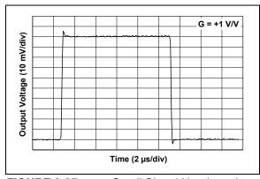
**FIGURE 2-27:** Small Signal Non-inverting Pulse Response.
