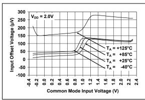
**FIGURE 2-3:** Input Offset Voltage vs. Common-mode Input Voltage, with  $V_{DD} = 2.0V$ .
