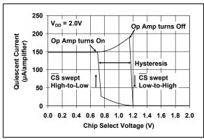
**FIGURE 2-25:** Quiescent Current vs. Chip Select  $\overline{(CS)}$  Voltage, with  $V_{DD}$  = 2.0V (MCP6273 and MCP6275 only).
