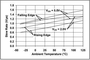
FIGURE 2-22: Slew Rate vs. Temperature.
