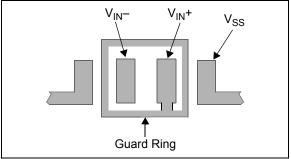
**FIGURE 4-7:** Example Guard Ring Layout for Inverting Gain.
