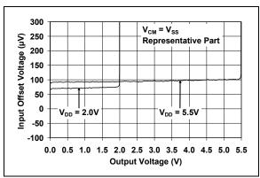
**FIGURE 2-8:** Input Offset Voltage vs. Output Voltage.
