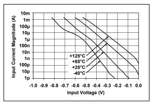
**FIGURE 2-32:** Input Current vs. Input Voltage.
