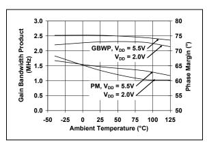
**FIGURE 2-18:** Gain Bandwidth Product, Phase Margin vs. Temperature.
