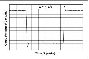
**FIGURE 2-30:** Small Signal Inverting Pulse Response.
