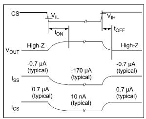
FIGURE 1-1: Timing Diagram for the Chip Select (CS) pin on the MCP6273 and MCP6275.
