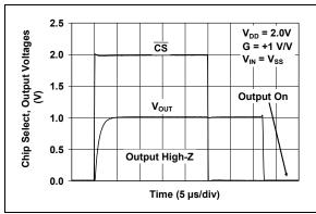
**FIGURE 2-31:** Chip Select ( $\overline{CS}$ ) to Amplifier Output Response Time, with  $V_{DD} = 2.0V$  (MCP6273 and MCP6275 only).
