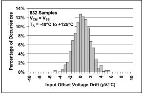
FIGURE 2-4: Input Offset Voltage Drift.
