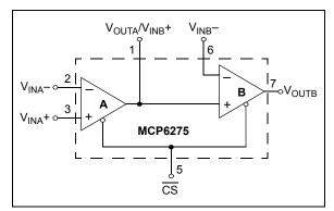
FIGURE 4-5: Cascaded Gain Amplifier.
