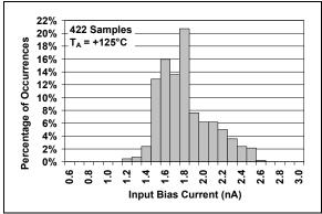
**FIGURE 2-5:** Input Bias Current at  $T_A = +125$ °C.
