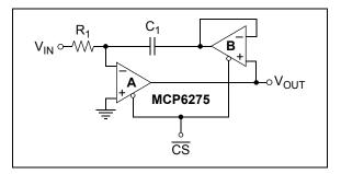
FIGURE 4-13: Integrator Circuit with Active Compensation.
