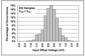
FIGURE 2-1: Input Offset Voltage.
