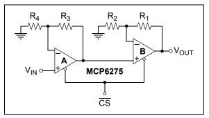
FIGURE 4-11: Cascaded Gain Circuit Configuration.
