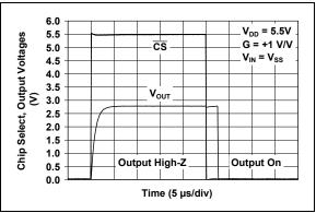
**FIGURE 2-33:** Chip Select  $(\overline{CS})$  to Amplifier Output Response Time, with  $V_{DD} = 5.5V$  (MCP6273 and MCP6275 only).
