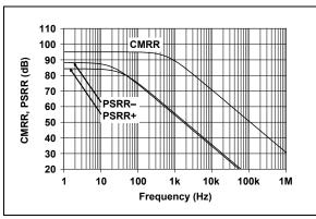
**FIGURE 2-9:** CMRR, PSRR vs. Frequency.
