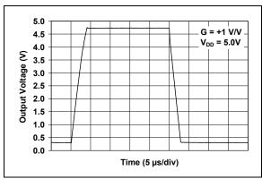
**FIGURE 2-26:** Large Signal Non-inverting Pulse Response.
