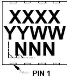
8-Lead DFN (3x3x0.9 mm) (MCP632)
