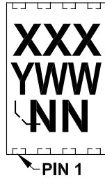
8-Lead DFN (3x3x0.9 mm) (MCP632)
