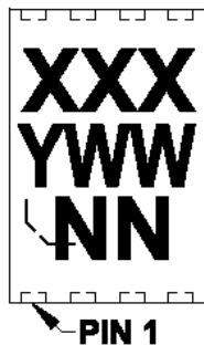
8-Lead TDFN (2x3x0.75 mm) (MCP6V67)
