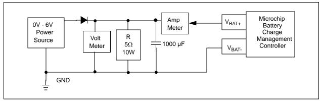
FIGURE 2-3: Simulated Battery Load.
