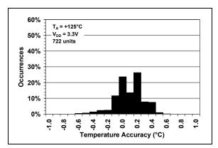
**FIGURE 2-5:** Temperature Accuracy Histogram,  $T_A = +125$ °C.
