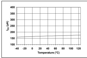
**FIGURE 2-7:** Supply Current vs. Temperature.
