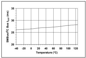
FIGURE 2-16: SMBus Timeout vs. Temperature.
