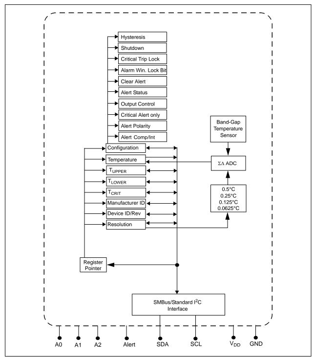
FIGURE 5-1: Functional Block Diagram.
