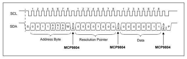
**FIGURE 5-9:** Timing Diagram for Changing  $T_A$  Resolution to 0.0625°C <0000 0011>b (See **Section 4.0**).
