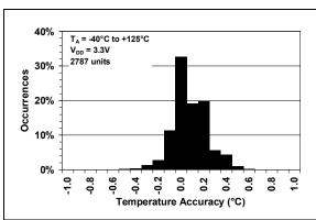
**FIGURE 2-2:** Temperature Accuracy Histogram,  $T_A = -40^{\circ}\text{C}$  to  $+125^{\circ}\text{C}$ .
