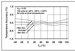
FIGURE 2-1: Temperature Accuracy.
