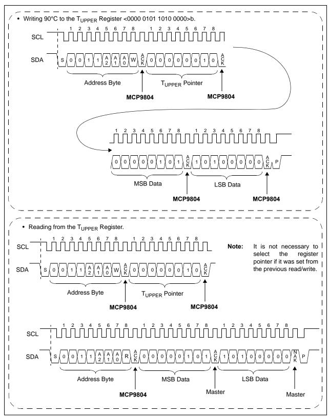
FIGURE 5-4: Timing Diagram for Writing and Reading from the T<sub>UPPER</sub> Register (See Section 4.0).
