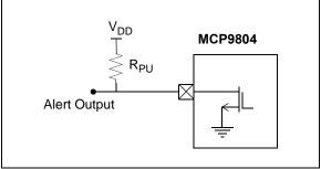
FIGURE 5-10: Active-Low Alert Output Configuration.
