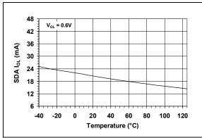
FIGURE 2-14: SDA I<sub>OL</sub> vs. Temperature.
