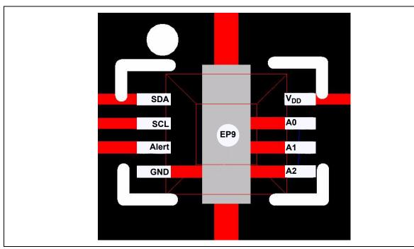
FIGURE 6-1: DFN Package Layout (Top View).
