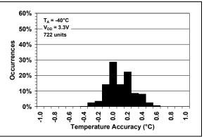
**FIGURE 2-6:** Temperature Accuracy Histogram,  $T_A = -40$  °C.
