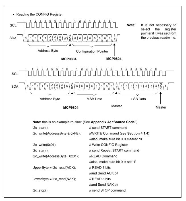
FIGURE 5-3: Timing Diagram for Reading from the Configuration Register (See Section 4.0).
