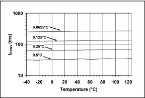
**FIGURE 2-12:** Temperature Conversion Time vs. Temperature.
