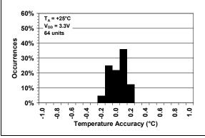
**FIGURE 2-3:** Temperature Accuracy Histogram,  $T_A = +25$ °C.
