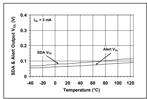
**FIGURE 2-13:** SDA & Alert output  $V_{OL}$  vs. Temperature.
