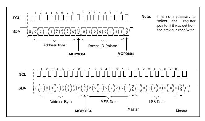
FIGURE 5-8: Timing Diagram for Reading Device ID and Device Revision Register (See Section 4.0).
