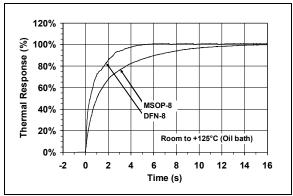
**FIGURE 2-15:** Package Thermal Response.
