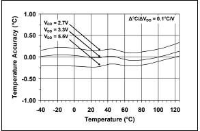
**FIGURE 2-10:** Temperature Accuracy vs. Supply Voltage.
