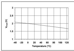
**FIGURE 2-9:** Power-on Reset Threshold Voltage vs. Temperature.
