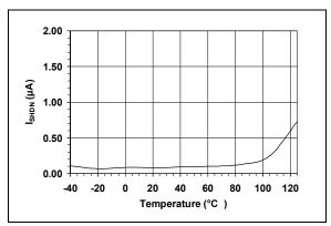
**FIGURE 2-8:** Shutdown Current vs. Temperature.
