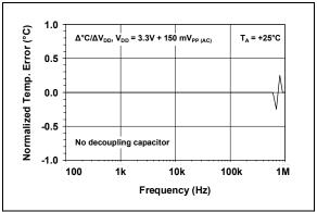
**FIGURE 2-11:** Power Supply Rejection vs. Frequency.
