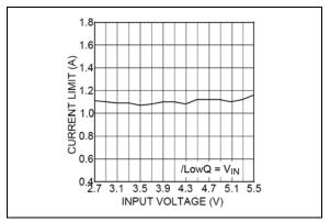
FIGURE 2-6: Current Limit vs. Input Voltage.
