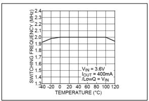
**FIGURE 2-3:** Switching Frequency vs. Temperature.
