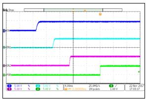
**FIGURE 2-34:** POR Behavior for Correct Sequencing.
