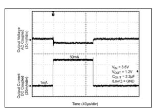
**FIGURE 2-25:** DC/DC (LOWQ Mode) Load Transient.
