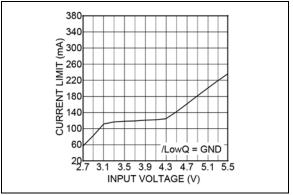
FIGURE 2-10: Current Limit vs. Input Voltage.
