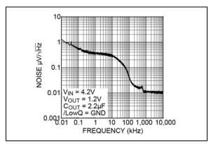
**FIGURE 2-11:** Output Noise Spectral Density.
