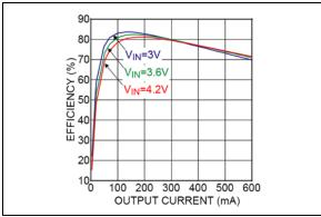
FIGURE 2-1: 1.2V<sub>OUT</sub> Efficiency.
