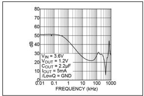
**FIGURE 2-7:** Power Supply Rejection Ratio.
