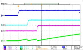
**FIGURE 2-33:** C<sub>SET</sub> Pin Voltage for Correct Sequencing.
