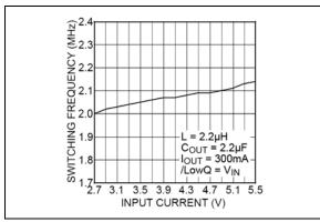
**FIGURE 2-2:** Switching Frequency vs. Input Voltage.
