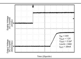
FIGURE 2-26: DC Start-Up Waveform.
