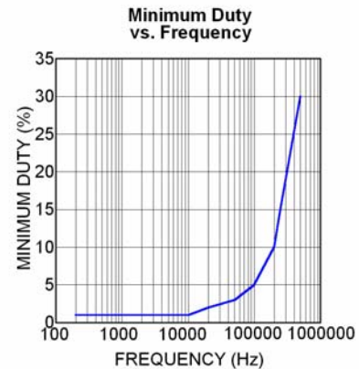
Figure 5. Minimum Duty Cycle for Varying PWM Frequency
