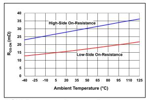
**FIGURE 2-5:**  $R_{DS(on)}$  vs. Temperature.
