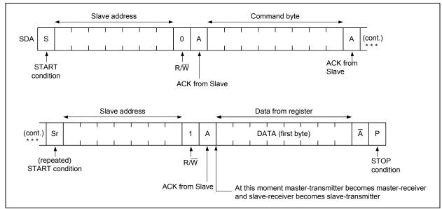
FIGURE 6-4: Single Read Timing Diagram.
