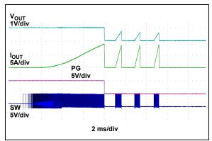
**FIGURE 2-24:** Output Current Limit Threshold.
