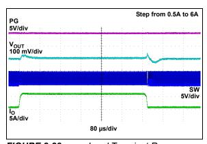
FIGURE 2-28: Load Transient Response.
