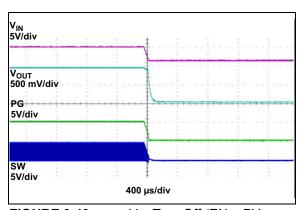
**FIGURE 2-19:**  $R_{IOAD} = 0.3\Omega$
