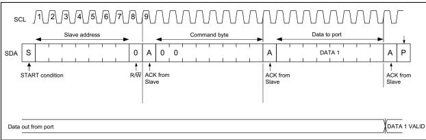
FIGURE 6-3: Single Write Timing Diagram.
