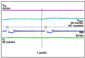
**FIGURE 2-26:** Switching Waveforms –  $I_{OUT}$  = 50 mA, HLL.
