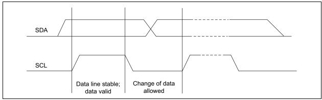
FIGURE 6-1: Bit Transfer Diagram.
