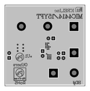
MIC4414/MIC4415 Evaluation Board – Copper Layer 2 (Bottom)
