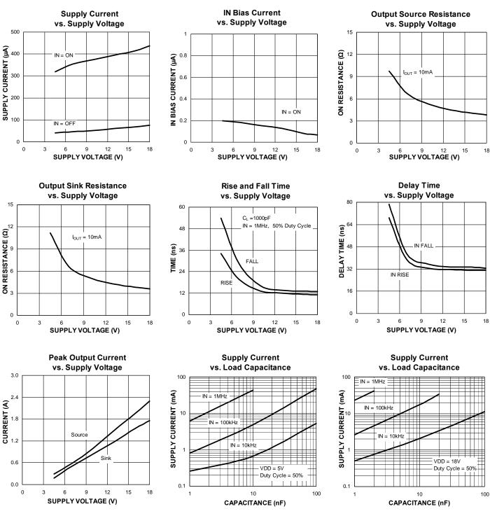
MIC4414/MIC4415 Evaluation Board Typical Characteristics
