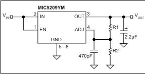
FIGURE 4-4: Ultra-Low-Noise Adjustable Application.
