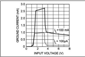
FIGURE 2-15: Ground Current vs. Supply Voltage.
