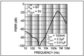
**FIGURE 2-6:** Power Supply Rejection Ratio.
