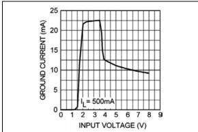
FIGURE 2-14: Ground Current vs. Supply Voltage.
