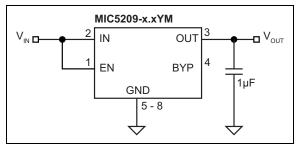
FIGURE 4-1: Low-Noise Fixed-Voltage Application.
