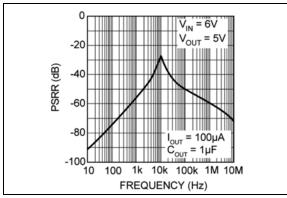
**FIGURE 2-1:** Power Supply Rejection Ratio.
