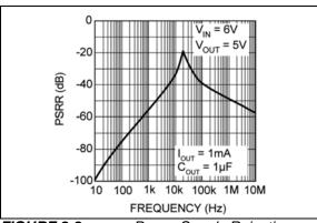
FIGURE 2-2: Power Supply Rejection Ratio.
