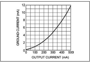
FIGURE 2-13: Ground Current vs. Output Current.
