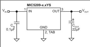
FIGURE 4-5: Slot-1 Power Supply.
