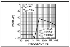
FIGURE 2-4: Power Supply Rejection Ratio.
