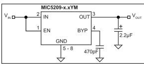
FIGURE 4-2: Ultra-Low-Noise Fixed-Voltage Application.
