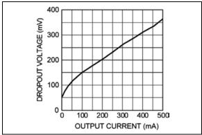
FIGURE 2-12: Dropout Voltage vs. Output Current.
