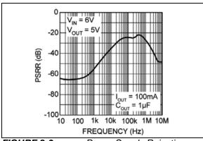
FIGURE 2-3: Power Supply Rejection Ratio.
