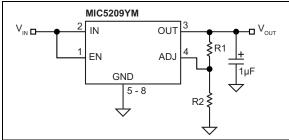
**FIGURE 4-3:** Low-Noise Adjustable-Voltage Application.
