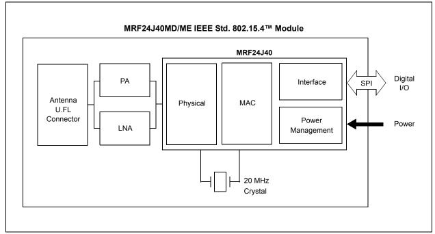
FIGURE 1-1: MRF24J40MD/ME BLOCK DIAGRAM
