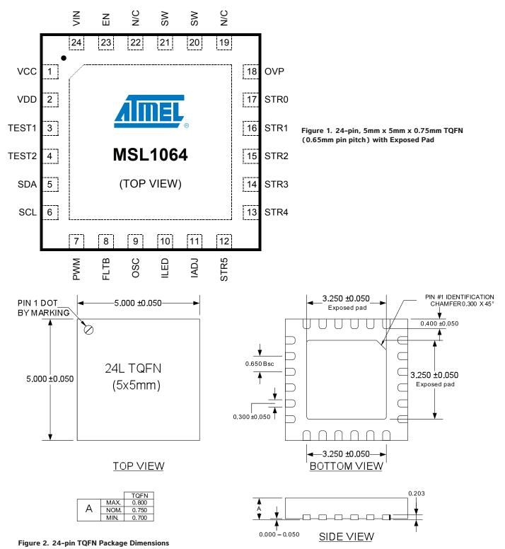
6-string PWM LED Driver with Digitally Compensated, 1.1MHz, 48V Boost Regulator, ±1.5% Current Balance, I<sup>2</sup>C Interface
