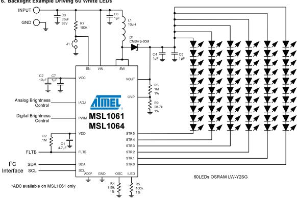
Figure 6. Backlight Example Driving 60 White LEDs
