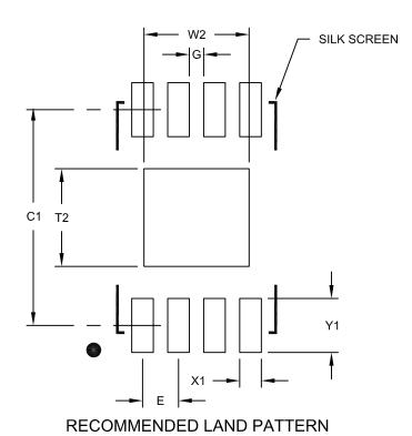
Units MILLIMETERS Dimension Limits MIN MOM MAX Contact Pitch Ε 0.50 BSC Optional Center Pad Width W2 1.46 Optional Center Pad Length T2 1.36 C1 Contact Pad Spacing 3.00 Contact Pad Width (X8) X1 0.30 Contact Pad Length (X8) <u>Y1</u> 0.75 Distance Between Pads G 0.20
