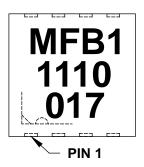
TABLE 30-1: 8-LEAD 2x3 DFN (MC) TOP MARKING
