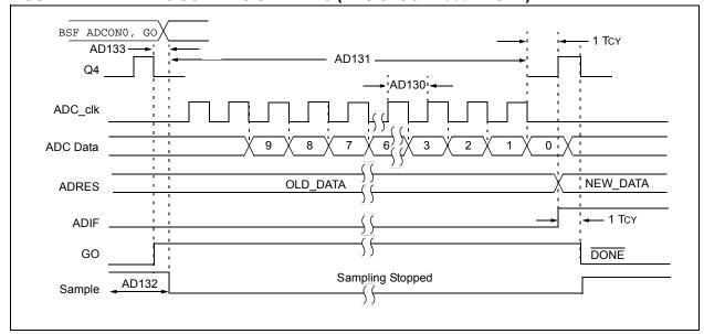
FIGURE 27-13: ADC CONVERSION TIMING (ADC CLOCK FROM FRC)
