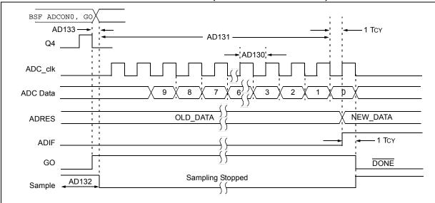
Note 1:If the ADC clock source is selected as FRC, a time of TCY is added before the ADC clock starts. This allows the SLEEP instruction to be executed.
