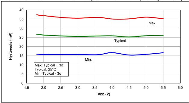
FIGURE 28-54: COMPARATOR HYSTERESIS, LOW-POWER MODE (CxSP = 0, CxHYS = 1)
