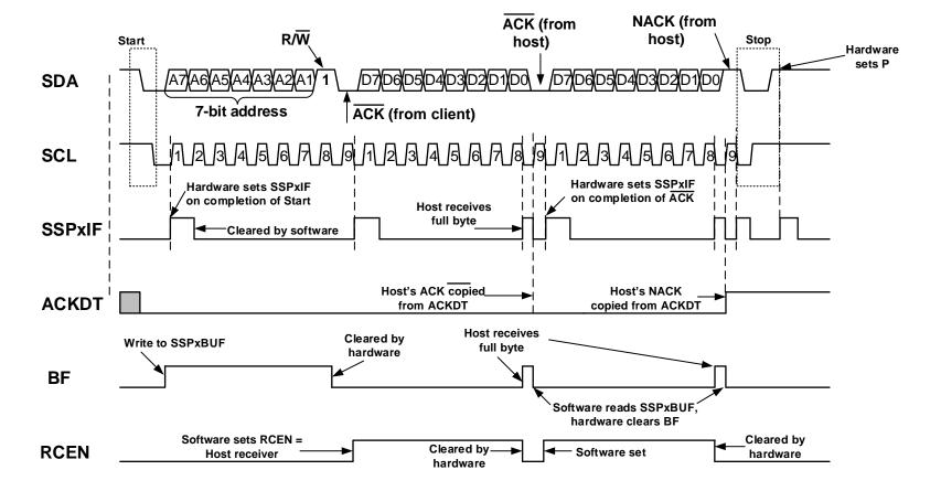
MSSP - Host Synchronous Serial Port
