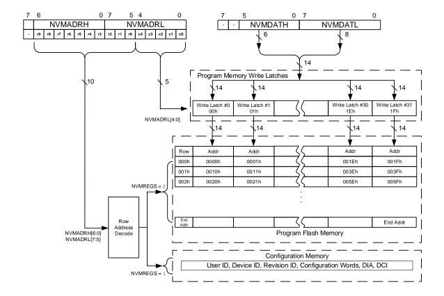
Figure 15-5. Program Flash Memory Write Sequence
