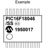
20-Lead SOIC (7.50 mm)
