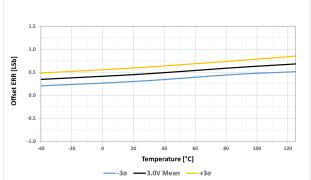
Figure 42-20. 8-BIT DAC, Absolute Accuracy vs. Temperature ( $V_{REF} = V_{DD} = 3.0V$ )
