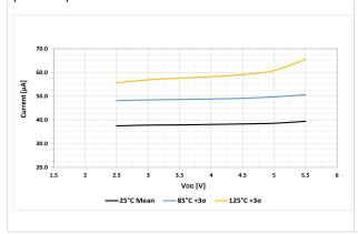
Figure 42-46. I<sub>PD</sub> Secondary Oscillator (SOSC)
