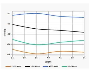
Figure 42-22. FVR Voltage Error vs. V<sub>DD</sub> 2x (V<sub>REF</sub> = 2.048V)
