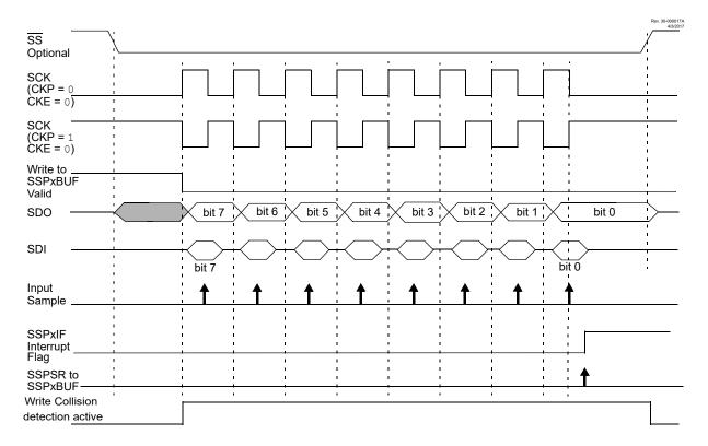
Figure 29-8. SPI Mode Waveform (Client Mode with CKE = 1)
