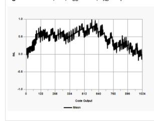
Figure 42-6. ADC, INL,  $V_{DD}$  = 3.0V,  $T_{AD}$  = 8  $\mu s$
