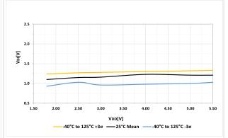
Figure 42-38. SMBus 3.0 Low Value ( $V_{IL}$  vs.  $V_{DD}$ )
