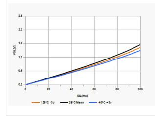
**Figure 42-55.**  $V_{OL}$  vs.  $I_{OL}$  over Temperature,  $V_{DD}$  = 3V
