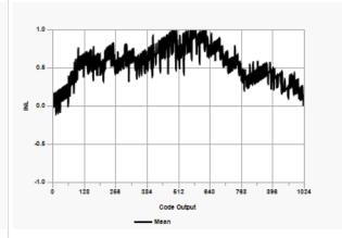
Figure 42-5. ADC, INL,  $V_{DD}$  = 3.0V,  $T_{AD}$  = 4  $\mu s$
