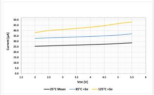
**Figure 42-42.** I<sub>PD</sub>, Comparator (SP = 1, CPON = 00)
