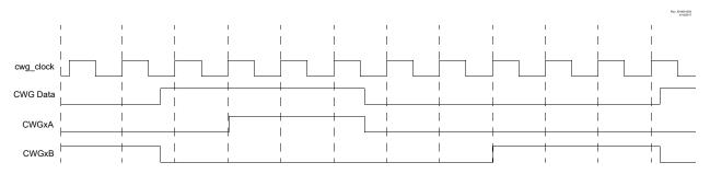
Dead band is always initiated on the edge of the input source signal. A count of zero indicates that no dead band is present.
