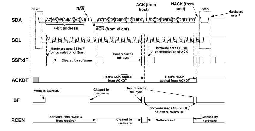
MSSP - Host Synchronous Serial Port
