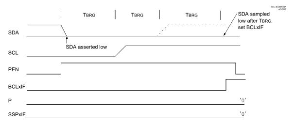
Figure 29-40. Bus Collision During a Stop Condition (Case 2)
