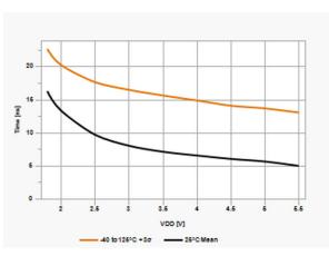
Figure 42-31. Fall Time, Slew Rate Control Disabled
