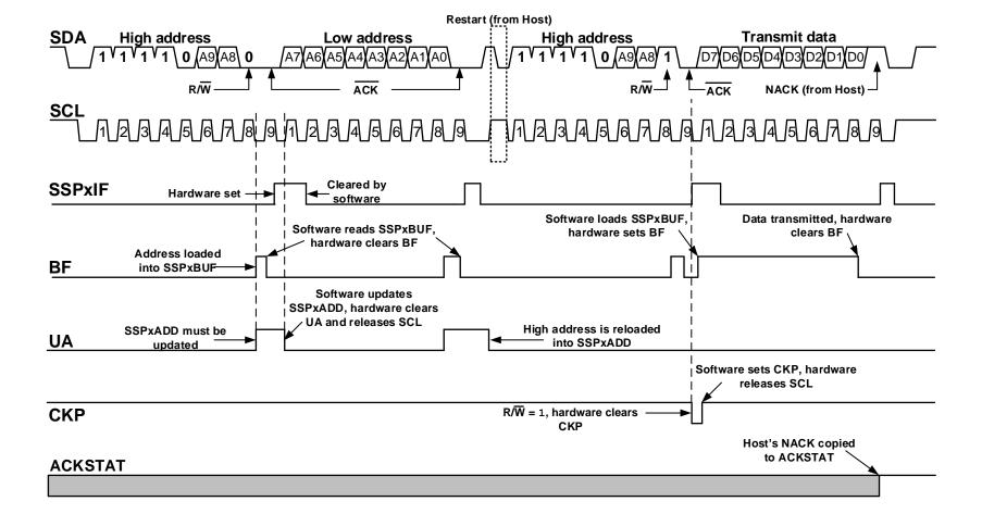
MSSP - Host Synchronous Serial Port
