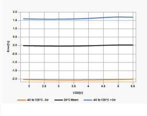
Figure 42-26. HFINTOSC Error % over Temperature, V<sub>DD</sub> = 3V
