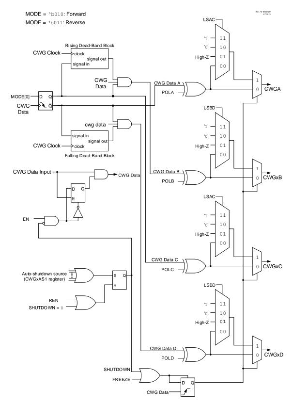
In Forward Full Bridge mode (MODE = <code>\b010</code>), CWGxA is driven to its Active state, CWGxB and CWGxC are driven to their Inactive state, and CWGxD is modulated by the input signal, as shown in Figure 23-7.
