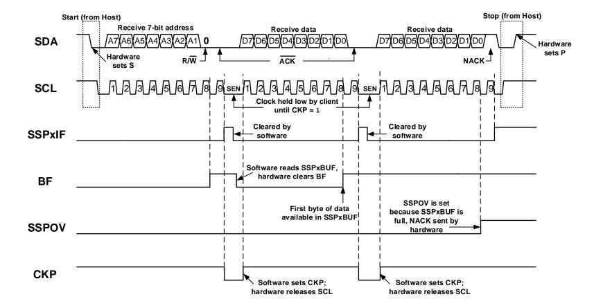
MSSP - Host Synchronous Serial Port
