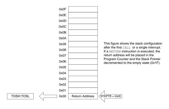
Figure 9-17. Accessing the Stack Example 3
