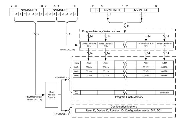
Figure 15-5. Program Flash Memory Write Sequence
