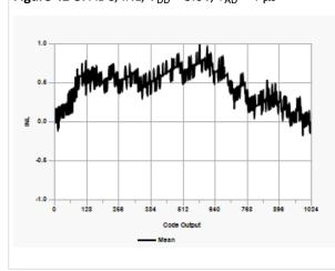
Figure 42-6. ADC, INL,  $V_{DD}$  = 3.0V,  $T_{AD}$  = 8  $\mu s$
