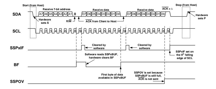
MSSP - Host Synchronous Serial Port
