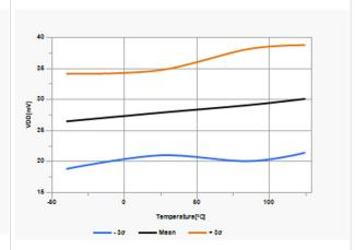
Figure 42-9. Brown-out Reset Voltage, Trip Point (BORV = 1)
