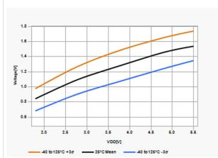
Figure 42-37. SMBus 3.0 High Value ( $V_{IH}$  vs.  $V_{DD}$ )
