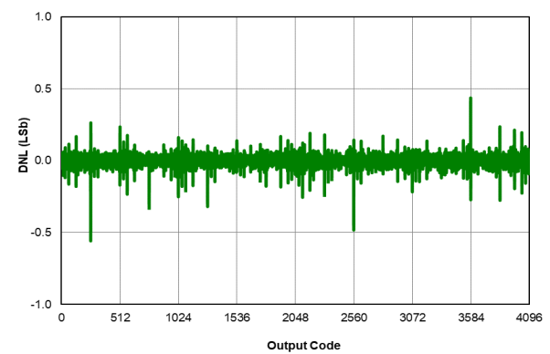
Figure 41-50. ADC 12-Bit Mode, Single-Ended DNL, V DD = 3.0V, V REF = 3.0V, T AD = 4 uS, 25°C, All devices
