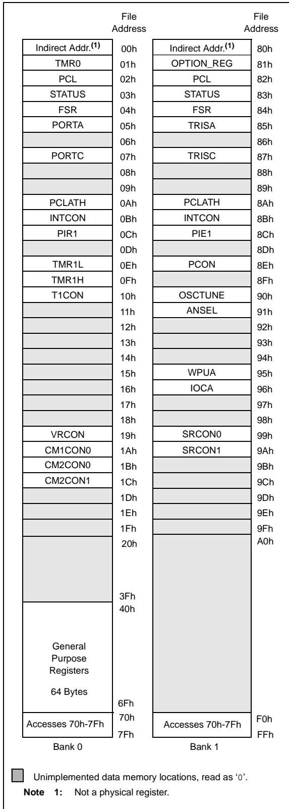
FIGURE 2-3: DATA MEMORY MAP OF THE PIC16F610/16HV610
