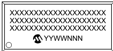
28-Lead SOIC (7.50 mm)
