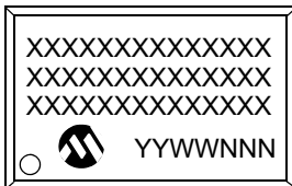
20-Lead SOIC (7.50 mm)
