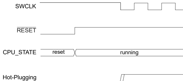
Figure 13-3. Hot-Plugging Detection Timing Diagram
