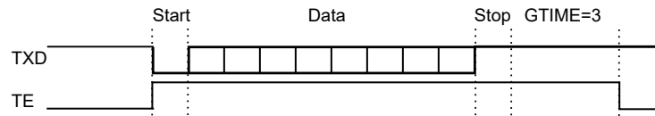
Figure 30-15. Example of TE Drive with Guard Time
