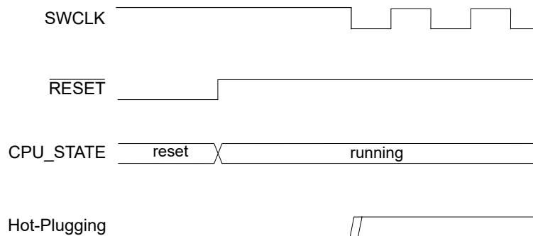
Figure 20-3. Hot-Plugging Detection Timing Diagram
