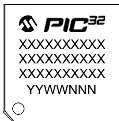
64-Lead TQFP (10x10x1 mm)
