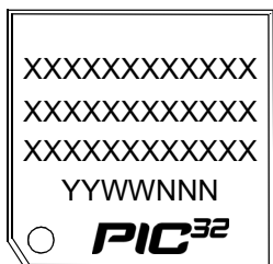
48-Lead VQFN (6x6x0.9 mm)
